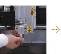
Attach the milling cutter best suited for the material and milling conditions. You can quickly set the origin on screen.
