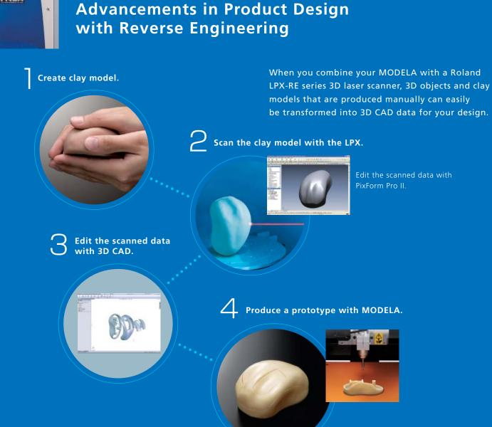
•Scans a wide variety of objects including hard surfaces and soft materials •Roland Pixform Pro II reverse modeling software is included and takes you from prototyping to the production process. Pixform Pro II generates lines, surfaces and models based on the data scanned with your LPX — data that can be used in 3D CAD software.
