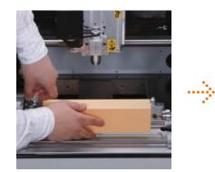
How you position the material differs depending on the shape of the material and your prototype design. The Rotary Axis Unit was used to produce this bottle prototype.
