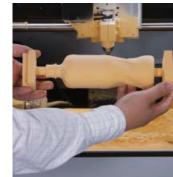
Once MODELA has finished milling, remove the part from the supports that secured the material to the unit and file the cut surfaces away.
