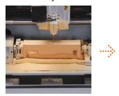
With the optional Rotary Axis Unit, objects can be milled unattended at any angle from 0 to 360 degrees and around multiple surfaces.
